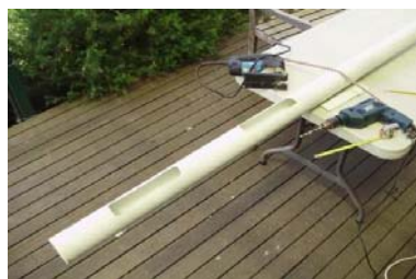
Photo 6, slots being cut.
