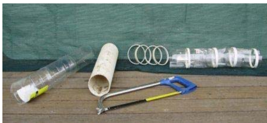
Photo 3. Bottles pushed into a pipe (left) and with PVC rings around the pipe (right) to stop it from being flattened.
